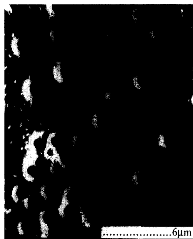
Figure 8 SEM micrograph of the ITO-facing surface of a PPy film prepared in 0.2M NapTS in 40/60 MeOH/H 2 O. Substrate: 15 Ωsq -1 ITO
